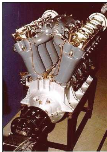
3a. A V8 engine with a 45° angle between banks
